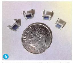
These photodiodes are essentially miniature solar cells.
