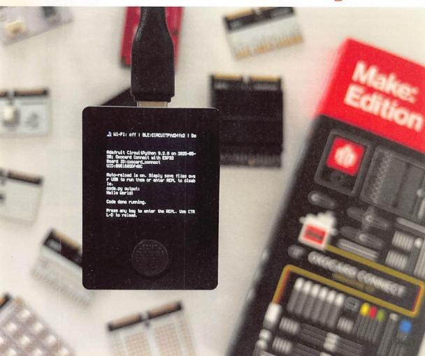
The Oxocard Connect is a versatile microcontroller board with a color display and plug-in cartridges for making all kinds of electronic projects. It has been designed to be programmed in NanoPv. a beginner-friendly language similar to Python, but you can also program it using CircuitPython, a popular Python implementation for microcontrollers. In this article we'll cover how to install CircuitPython, the basics of programming with it, and some simple experiments to get you started.
