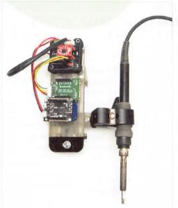
SOLDERING IRON ELECTRONICS: an off-theshelf "backpack motor driver" (top) and ESP32 microcontroller board (a TTGO T7, bottom), and my own "Betsy" single-axis CNC module.
