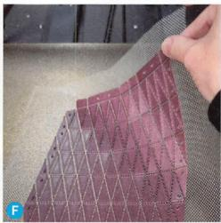
no tape covers any of the 3D-printed shapes. Press the tape down gently but firmly so that it is completely flat, being careful not to move the printer bed or the extruder. Then resume the print using your printer's controls.
