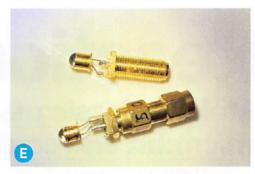
While the component connected to an SMA connector resembles a standard photodiode, it is actually an LED used as a narrow-wavelength photodiode.
