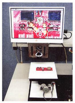
MICROSCOPE STAGE: A macrophotography tripod head has been repurposed, with the addition of a deck plate and some motors salvaged from dead printers. as an X-Y microscope stage.
