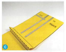
the lines of conductive tape. When you press a button, it connects the lines of tape and closes the circuit. This allows some electricity to flow between the micro:bit pin that the button is attached to (pin P0, P1, or P2) and the Ground pin (GND). The micro:bit registers the increase in voltage as input - the same way it would if you pushed one of the on-board buttons - which triggers a bit of code that shows who hit their button first and won the round!
